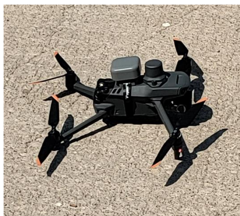
Figure 4: Drone used to survey the campus and create the 3D map
