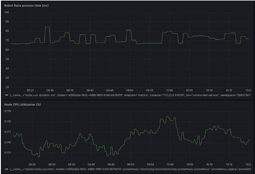
Figure 33: Cloudlet CPU utilization (bottom) and the corresponding response time of the Robot Race App (top)
