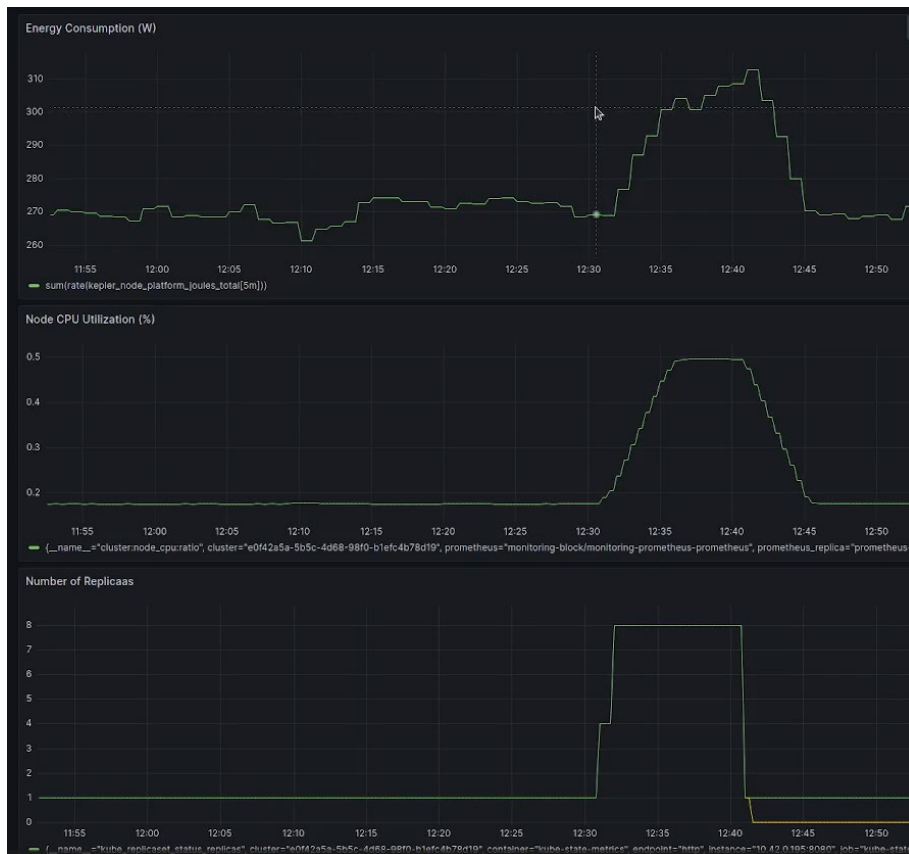
Figure 43: Grafana dashboard monitor for the node CPU utilisation, Energy consumption and number of application replicas
