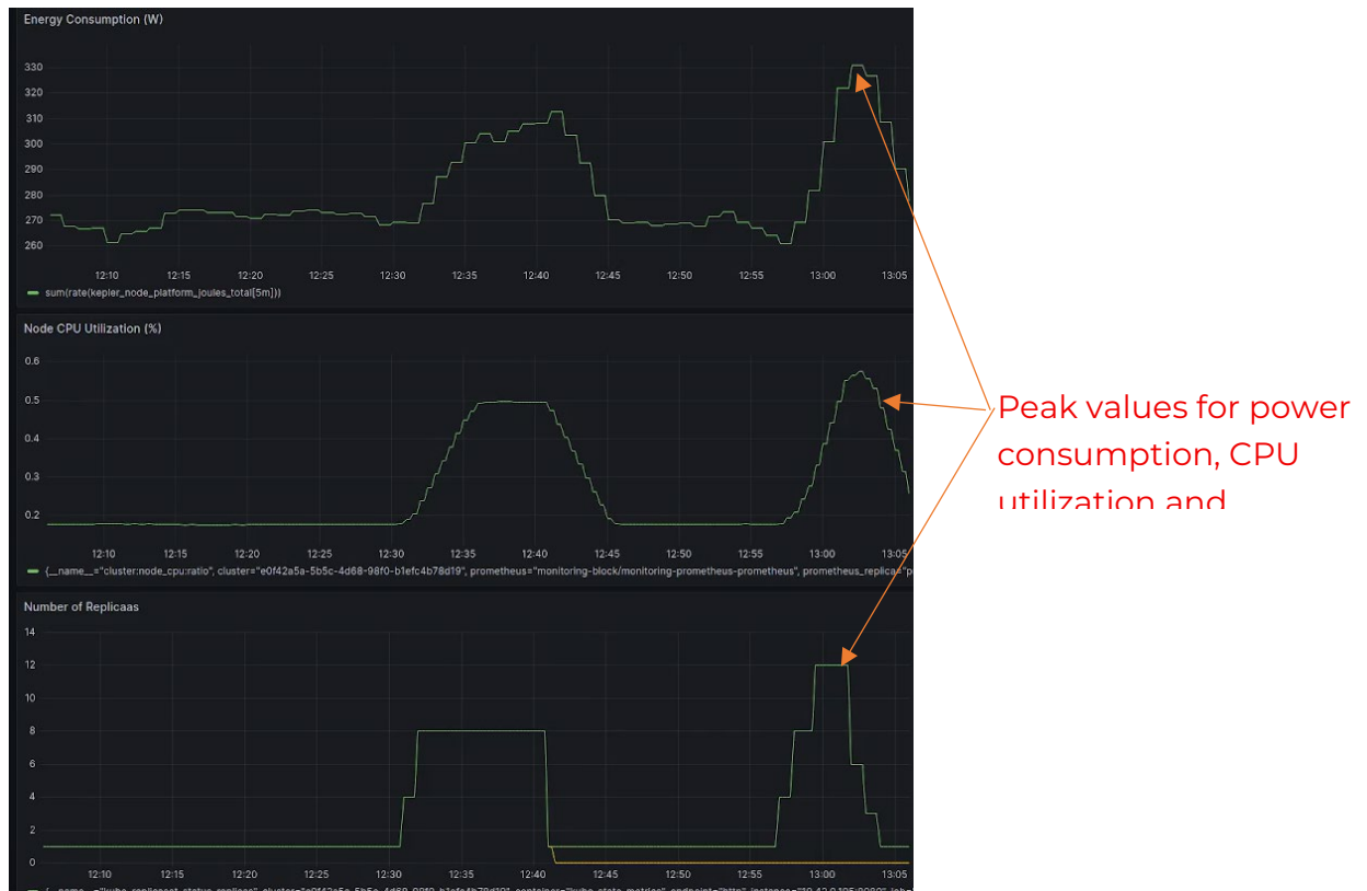
Figure 46: Power consumption normalisation
